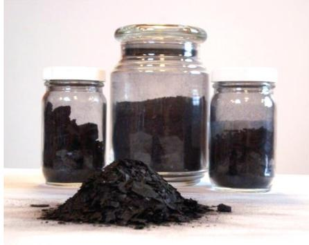
**Figure 3:** Photo of Bio-Char Produced by MAGS™
