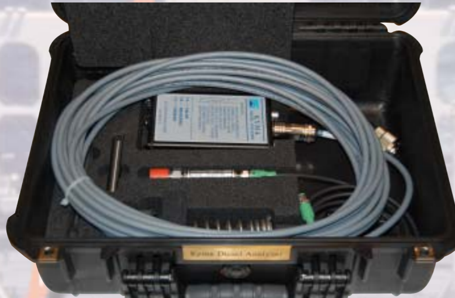
Picture show the transportation suitcase with sensors.
