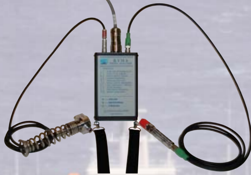
Figure shows the hand held unit with both cylinder pressure sensor and fuel injection pressure sensor.
