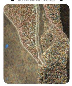
The robust circulation creates a sloughing effect on the thick biomass growth...eliminating the need for any media maintenance.
