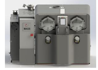
MAGS generates 70 kWh of energy in hot water from about 40 kg of mixed waste every hour.
