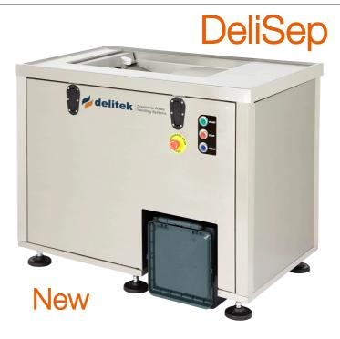
A DeliSep FW Processing Station consists of a macerator followed by centrifugal treatment of the food waste slurry.
